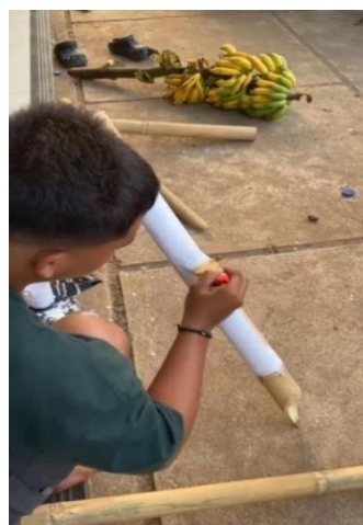
Figure 3. Painting process of the bamboo delineator structure
