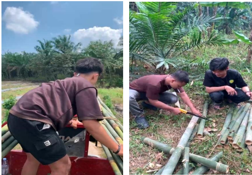
Figure 2. Process of transporting bamboo from the plantation using a three-wheeled vehicle and cutting the bamboo to the required sizes.
